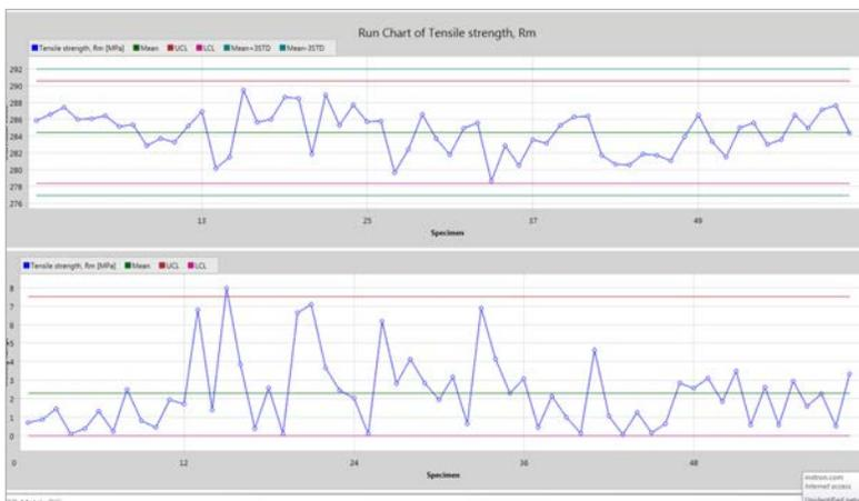
An Xbar-R Chart with Control and Specification Limits
