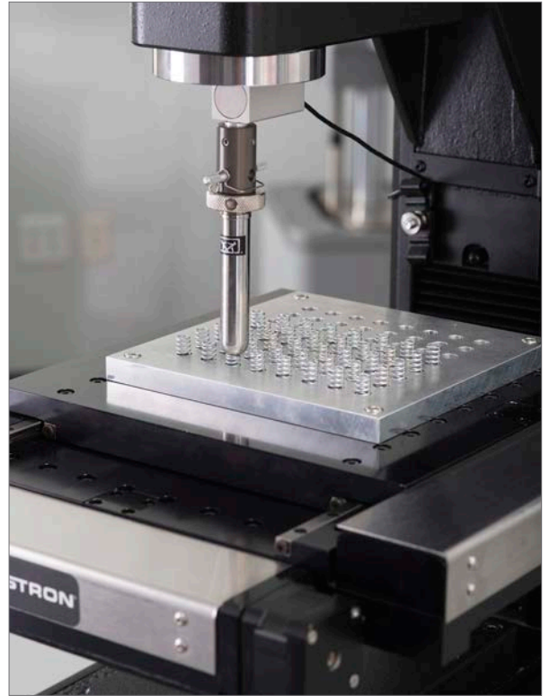
Compression Testing on Springs used in Surgical Equipment
